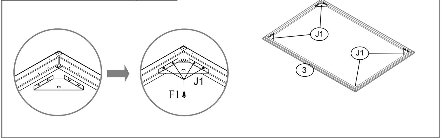
1. When diagonal measurements are equal, the frame is square.
