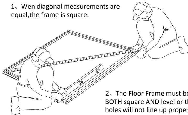
2. The Floor Frame must be BOTH square AND level or the holes will not line up properly.
