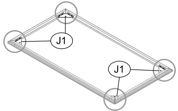
1. When diagonal measurements are equal, the frame is square.
